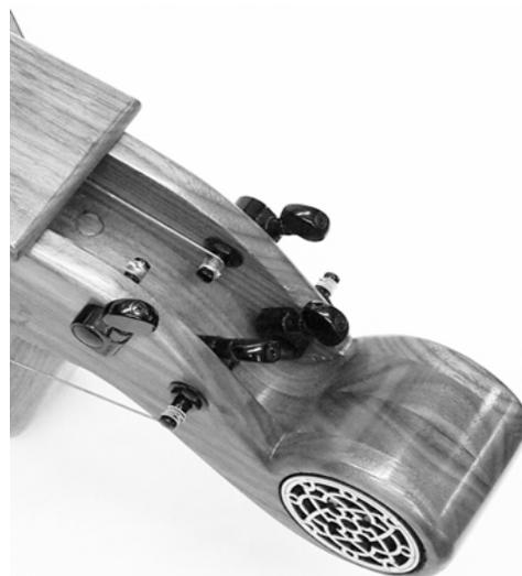
\_\_\_\_\_ **46.** Use a 1/16” bit to drill a small hole near the point of each **DRONE NUT** so the drone strings can be threaded through the holes.
