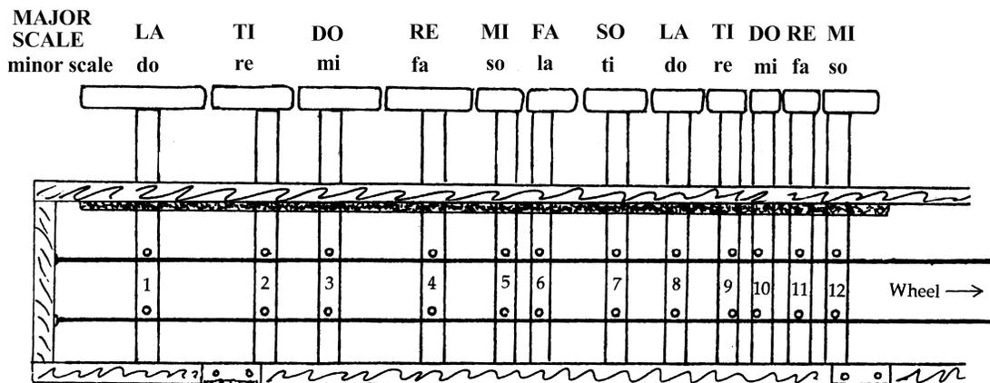
If any notes sound out of tune, you can correct the pitch by turning the **TANGENTS** inside the **KEYCHEST**. Turning them toward the **WHEEL** will raise the pitch, and vice versa. Make sure to adjust both **TANGENTS** on a key identically, so they make the two melody strings sound the same pitch.
