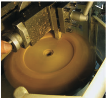
turn the face to correct taper
