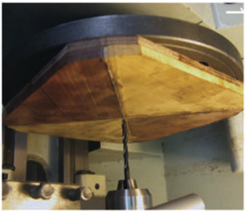
Glue the quarters of contrasting woods (huon and blackwood) to the hardwood plywood core. This is then attached to the lathe faceplate
