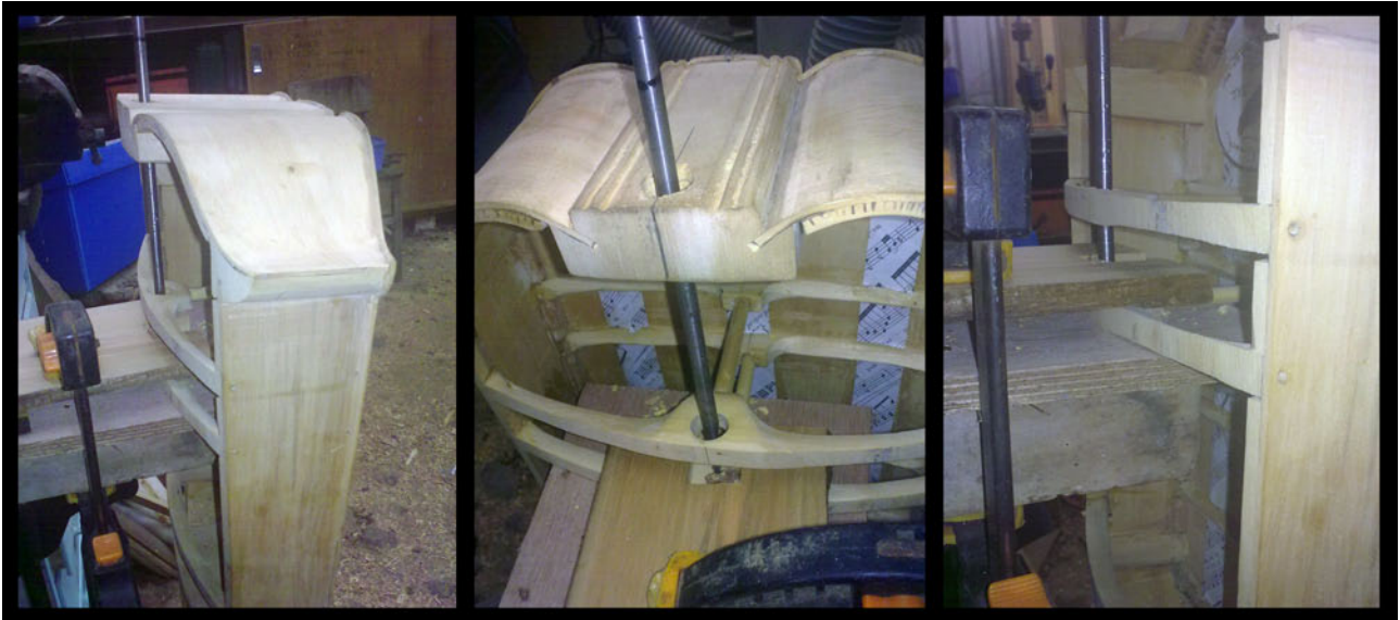
Drilling the axle holes
