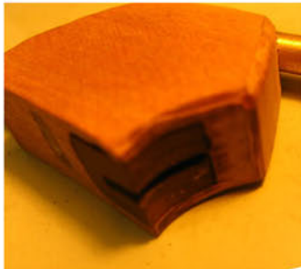
showing the ebony slider. This is what the dog will pivot on
