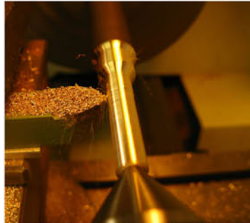
Turning the shaft of the bolt
