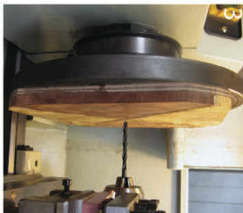
Centre the pilot hole drill and check that it is exactly 90° to the wheel face. Now drill the pilot hole
