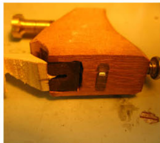
the adjustable dog bridge com- ponents in place
