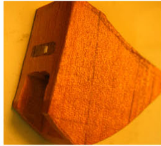
Route out the adjustable slider slot and inbed the adjuster nut
