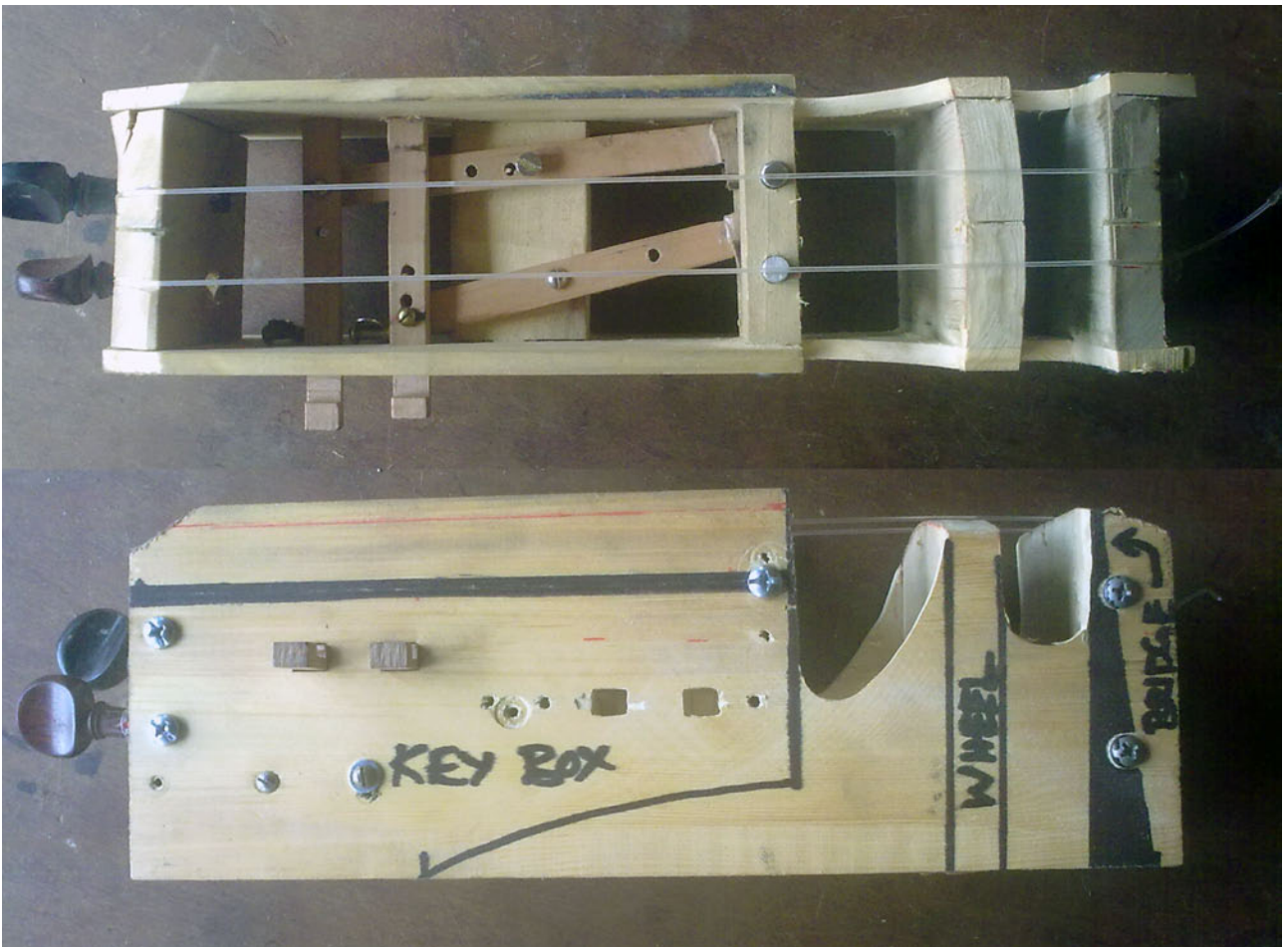
Showing the "mock up" of the Chanter string lifters
