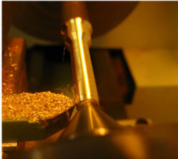
Turning the shape to the adjustable bridge bolt out of brass. The is one for each of the drones (Alto, Tenor & Bass)
