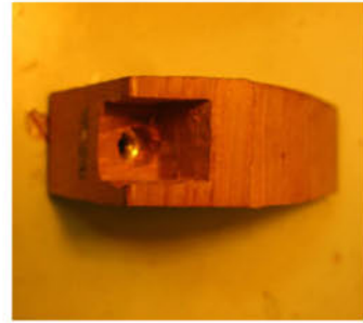
Showing the adjustable slider slot and adjuster bolt hole
