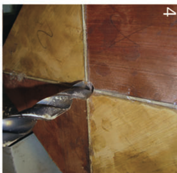
Now drill the 2mm deep wheel thread flange seat. ie. the largest diameter of the wheel thread.
