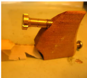
showing the dog blank getting fitted to the slider slot. also showing the Alto bridge bolt
