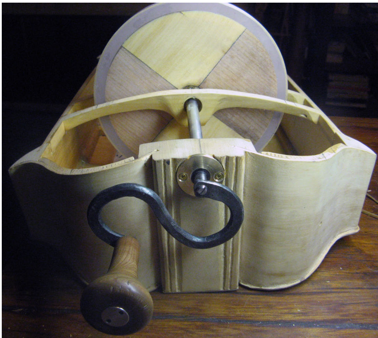
The wheel and shaft installed. This photo shows the clearance of the bridge brace to the shaft.
