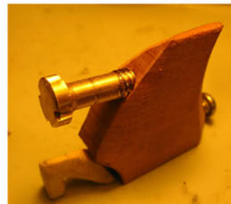
the alto bridge bolt. It screws in and out for adjustment
